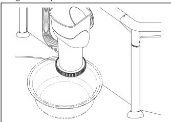
d. Remove the Top Cover, Strainer Basket, and Filter Cartridge. Use a water container (e.g. a bucket, not
