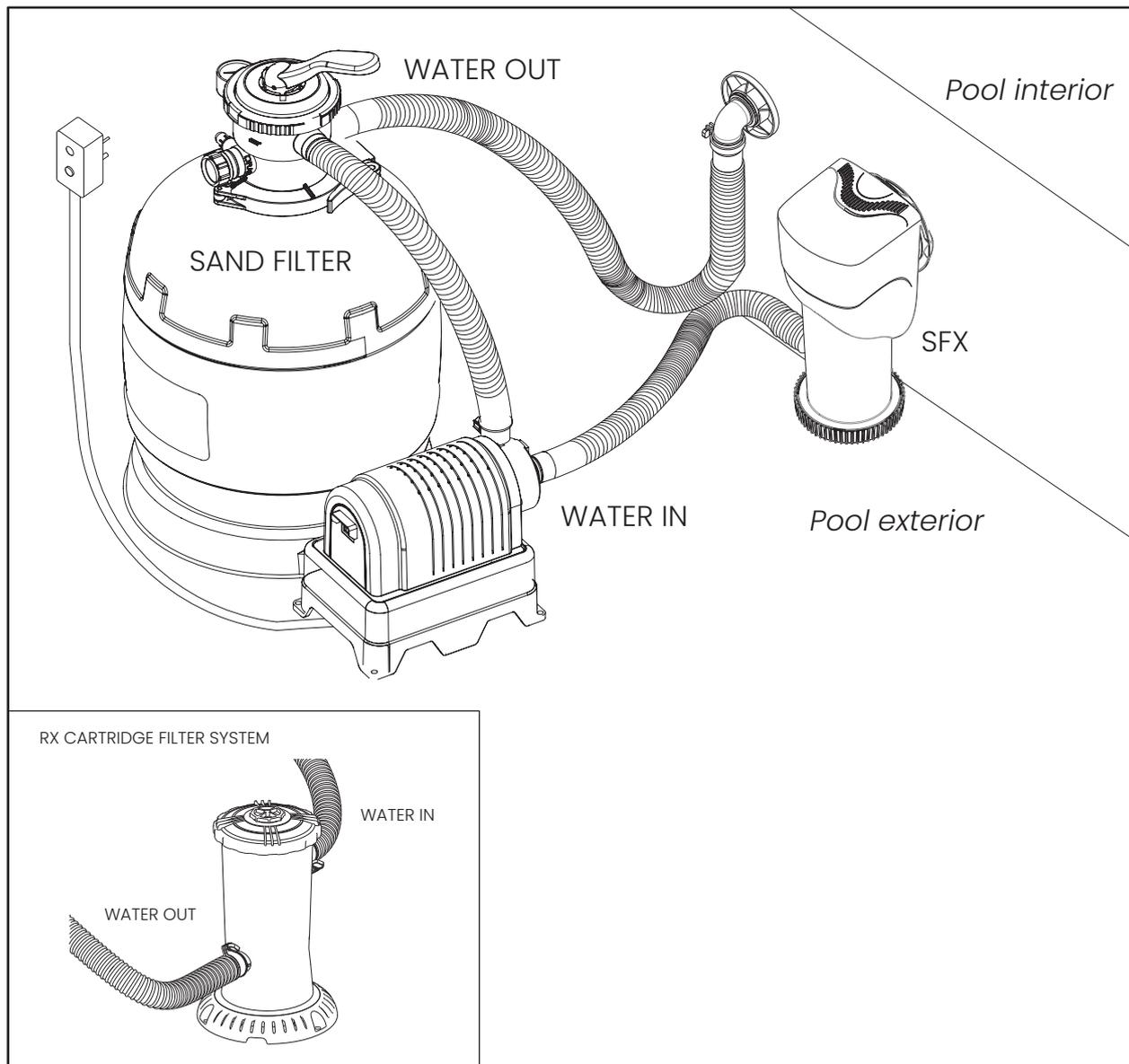
5. Refer to the instruction user guide and make sure that all connections are firmly secured.
