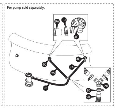
Make sure the Hose Clamps **①** seal tightly over both the Hose **③** and O-Rings **②**.
