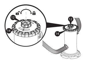
c. Using both hands, twist counterclockwise to remove the Seal Top 2.
