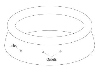
3. From inside the pool, install the Return Fitting **6** into the Inlet opening.
