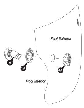
2. Install the Suction Fitting components into the Outlet opening.
