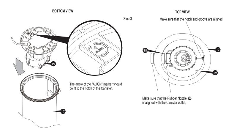
4. Once the Motor is correctly aligned, and the Canister Gasket is in place, match the threads of the Pump Base to that of the Canister, and tighten by twisting the Base clockwise.
