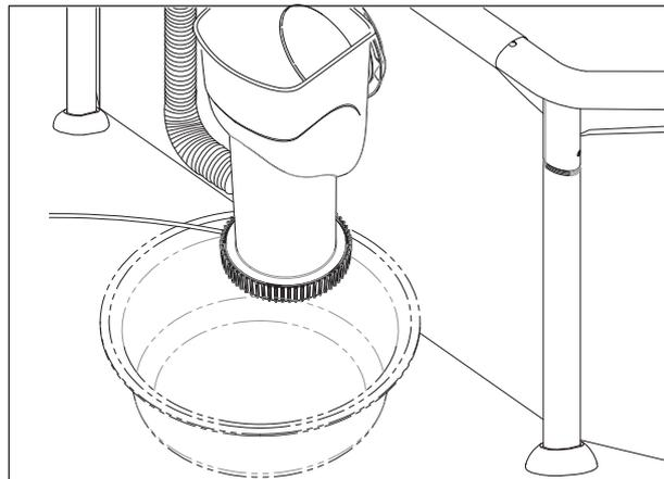
4) Remove the Top Cover, Strainer Basket, and Filter Cartridge. Use a water container (e.g. a bucket, not included) to collect the purged water resulting from servicing the pump.
