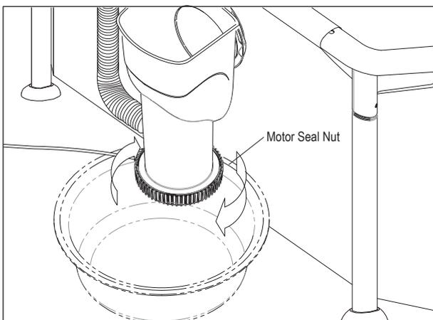
5) Remove the Motor Seal Nut by turning it clockwise. Do not pull or push the canister, as this can cause damage between the canister and pool liner.
