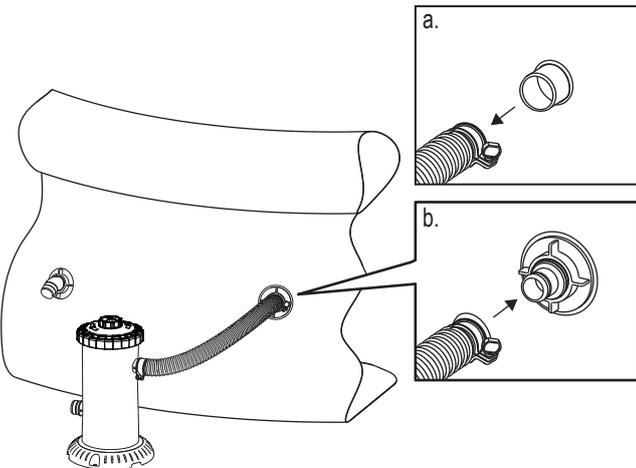
4) Tighten the Hose Clamps to prevent loosening and water leakage. Repeat steps 2, 3 & 4. Connect the Return Fitting to the Filter Pump Outlet (sequence as shown below).
