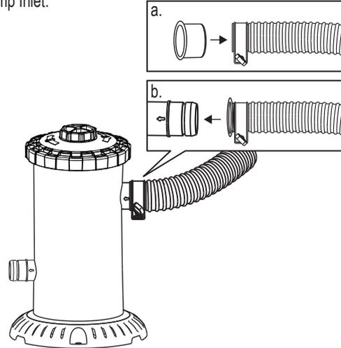
3) Insert another Hose Adapter to the other end of the hose and then, connect the hose to the Suction Fitting of the pool.
