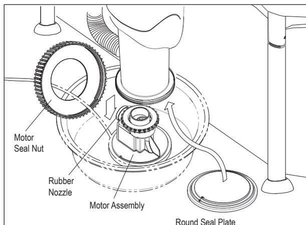
6) Remove the SFX Motor Assembly, and seal the Canister opening with the Seal Plate. Fasten the Motor Seal Nut tightly to ensure that no water leaks.
