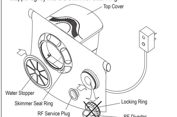
3) Detach the Locking Ring and RF Diverter by turning it counterclockwise. Insert the Service Plug.
