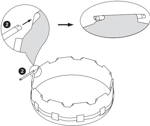
9. Connect all of the T-Fittings **4** to the Horizontal Beams **2**.
