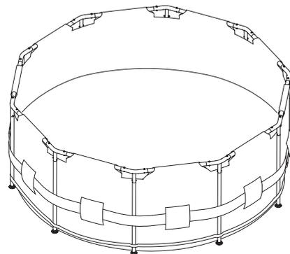
14. Fill up the pool with about an inch (1") [2.54cm] of water. Stop filling and smooth out all wrinkles from the pool floor, working outwards from the center, so that it fills evenly.
