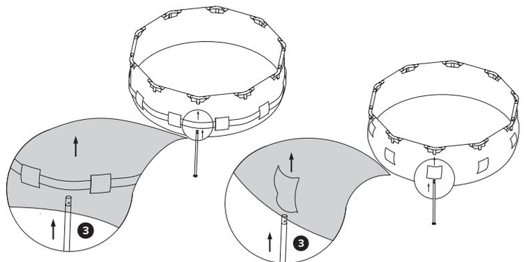
12. Look through the hole in the T-fitting, as you insert the Vertical Leg rotate it until the buttons align with the holes and pop out, locking the Vertical Leg in place. Do this for all Vertical Legs.
