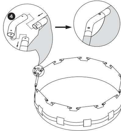
10. Insert the Pins **6** down through the top of the T-Fittings until the Pins snap into place on the lower side of the T-fitting.
