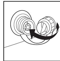
c) Flip the drain cap and reinsert it to the drain valve
