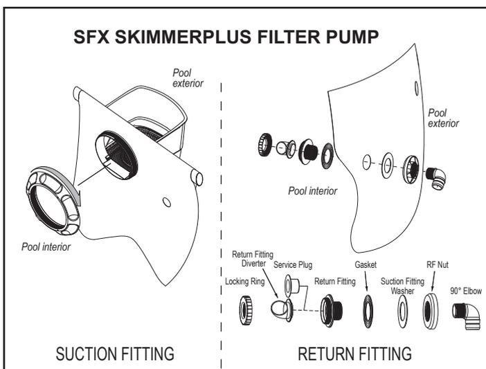
**NOTE:** For Sand Filter Pump / Cartridge Filter Pump CP2000-C, please follow the Sand Filter Pump / Cartridge Filter Pump CP2000-C owner's manual to set up the fitting. Please check the water pump's instruction manual for more instructions.
