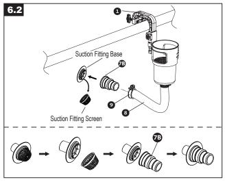
If the Suction Fitting of your pool is the same type as illustrated in **6.2**, remove the Suction Fitting Screen from the Suction Fitting Base first. Attach the Adapter **1** to the Suction Fitting Base and fix tightly.
