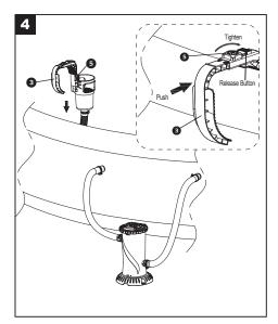
Hang the Ring Pool Surface Skimmer onto the top inflatable ring of the ring pool and then loosen the Lock Nut ③ in anti-clockwise by hand. Push the Ring Pool Holding Frame to fix the Ring Pool Surface Skimmer on the ring pool. (Push the Release Button to loosen the Ring Pool Holding Frame Rear ③ ).
