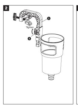
Turn the Lock Nut **5** in clockwise to tighten the Frame Pool Holding Frame **1** by hand.
