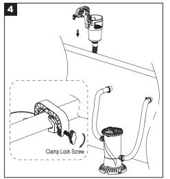
Hang the Frame Pool Surface Skimmer onto the top pole of the frame pool and then turn the Clamp Lock Screw in clockwise to tighten the Skimmer by hand.
