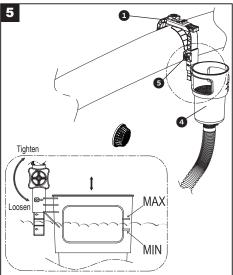
Loosen the Lock Nut (5) in anti-clockwise by hand and adjust the position of the Skimmer Canister (1) on the Ring Pool Holding Frame. The position of the Skimmer Canister (1) should be set as the pool water surface between the water level marking on the Skimmer Canister (1). Tighten the Lock Nut (5) in clockwise to hold the Skimmer Canister (4) in your setting position.
