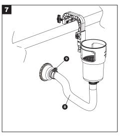
Then, connect the Hose (3) to the adapter, and tighten the Hose Clamp (9).
