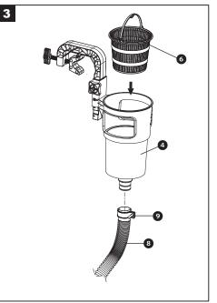
Insert the Skimmer Basket (6) into the Skimmer Canister (4). Connect the hose into the hose connector on the bottom of the Skimmer Canister (4) and fasten the hose by hose clamp.
