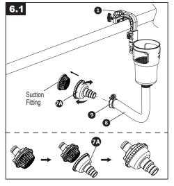
If the Suction Sitting of your pool is the same type as illustrated in **6.1**, attach the Adapter **2** to the Suction Fitting and screw tightly.
