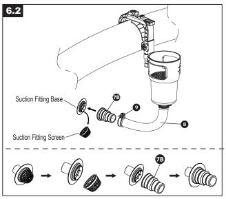
If the Suction Fitting of your pool is the same type as illustrated in **6.2**, remove the Suction Fitting Screen from the Suction Fitting Base first. Attach the Adapter 😰 to the Suction Fitting Base and fix tightly.
