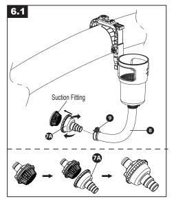
If the Suction Fitting of your pool is the same type as illustrated in **6.1**, attach the Adapter **2** to the Suction Fitting and screw tightly.
