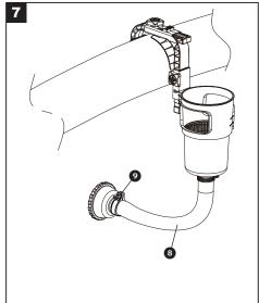
Then, connect the Hose (3) to the adapter, and tighten the Hose Clamp (9).
