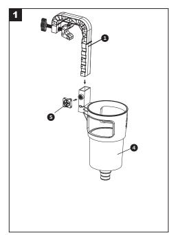
Insert the Frame Pool Holding Frame 1 into the Skimmer Canister 4. Put the Lock Nut 5 onto the screw hole of the Skimmer Canister 4.
