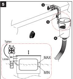
Loosen the Lock Nut (5) in anti-clockwise by hand and adjust the position of the Skimmer Canister (1) on the Frame Pool Holding Frame (1). The position of the Skimmer Canister (1) should be set as the pool water surface between the water level marking on the Skimmer Canister (1). Tighten the Lock Nut (5) in clockwise to hold the Skimmer Canister (4) in your setting position.
